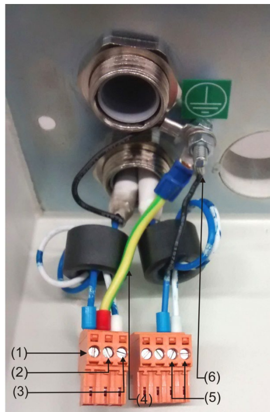
Figure 11: Power and signal connections to the docking station
