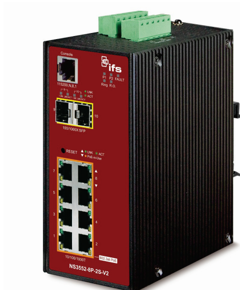
Figure 1: NS3552-8P-2S-V2 Industrial L2+ Multi-Port Managed Ethernet Switch
