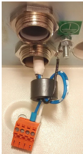
Figure 7: Looping relay connection wires around a suppression ferrite
