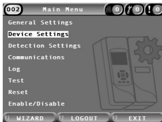
Figure 24: Access level 3 Main menu
